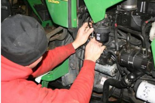
Mark Clem (left) is replacing the fuel line in the 5210 John Deer Tractor that mows and maintains the course roughs.
